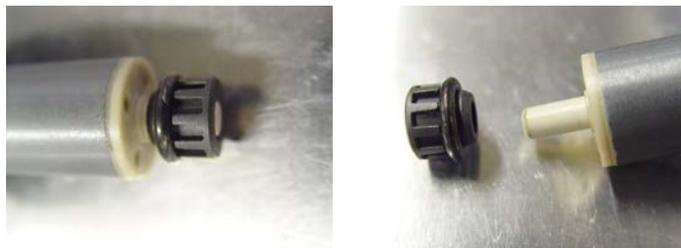
If the rear bearing brush – as seen on the photo – sits on the shaft when removing the impeller unit, it is vital to carefully remove the bearing from the shaft photo
