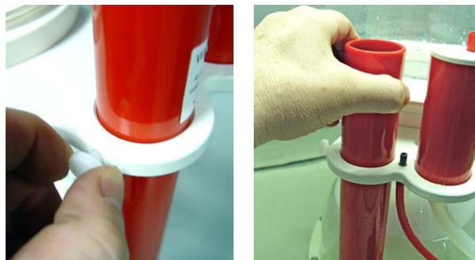
There is a small screw at the edge of the wedge shaped tube holder with which the wedge shaped tube can be clamped into the guide holder.
