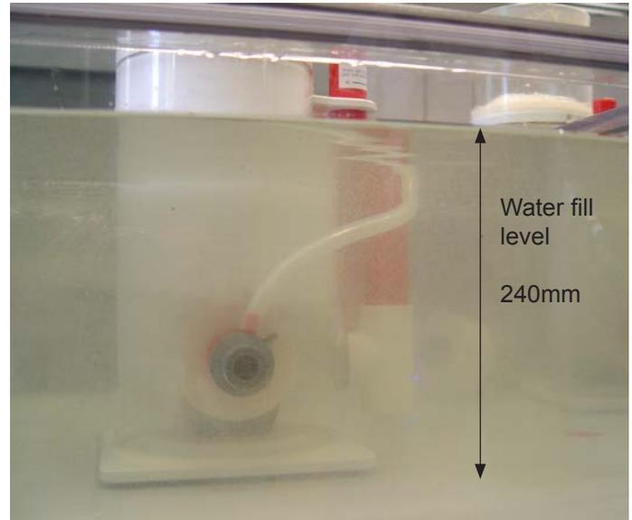
Depending on how high is the water fill level in the filter, the Bubble King® Double Cone can be placed on the right height, to achieve an optimal result of skimming.
