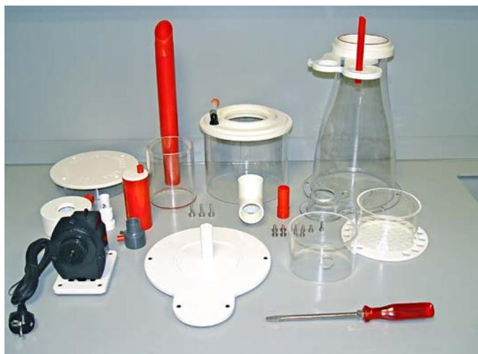
Remove all parts which can be dismantled, such as the wedge shaped tube, pot, hose, pump and also the T-piece from the outlet, including all titanium screws. Pull out the red pipe for injection using a sharp tong.
