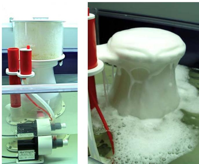
Let the skimmer run for several hours without placing the pot on top.
