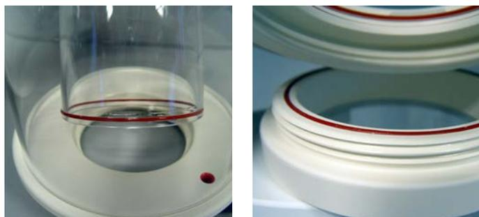
Regular lubrication with silicon grease enables easy rotation of the thread. The foam tube can be removed. After cleaning, lubricate or wet the O-ring. Push it against the notch and press down with a gentle rotation.
