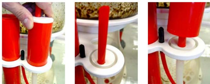
Clamping the resonator
