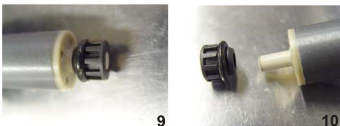
Impeller units where the bearing is firmly bonded to the shaft must not be under circumstance reinserted into the pump. Blocked bearings may cause damage to the pump or prevent it starting up, due to the O-ring grinding against the bearing seat.
