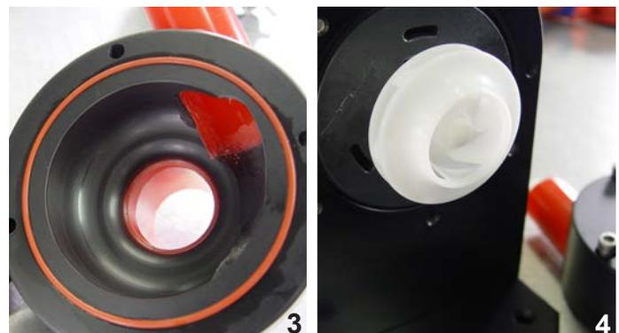
For assembly (fig. 1-8): fix the O-ring in position, then carefully let the magnetic impeller with the lip on top click into place. Caution ! **Strong magnetic forces !!**
